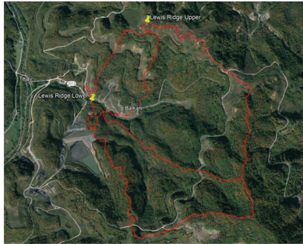
Drainage Area of Preliminary Lower Reservoir
